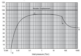
Actual performance curve will depend on the booster model, the backing pump performance curve, and additional factors.
